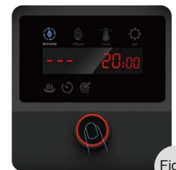
3. In Activating, when setting-temp. is reached, the infuser starts the timer(Fig.4), press the Dial to Pause or Restore Activate Mode(Fig.5). The timer stops, the infuser returns to standby mode and reads out "OFF"(Fig.1).
